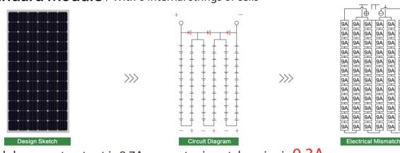
Module current output is 8.7A, current mismatch series is 0.3A.
