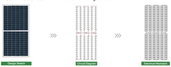
Module current output is 4.5+4.35=8.75A, current mismatch series is 0.15A.
