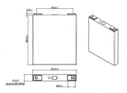
It adopts 3.2V/105Ah lithium iron phosphate battery independently developed and produced by Shanghai Electric Guoxuan, which has four major features such as high safety, long cycle life, superior multiplier charging and discharging performance, green and pollution-free, etc. Its main technical parameters are as follows.
