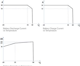
Battery Capacity vs Temperature (Discharge from 57.5V to 40V, 0.2C, 100% DOD)
