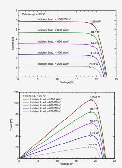
STC: Irradiance 1000W/m<sup>2</sup>,Module temperature 25°C, AM1.5 spectrum.
