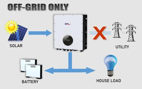
In this operation mode, grid feedback to utility is disabled. Users can only program unit to:
