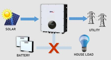
In this operation mode, the inverter will only behave like a pure grid-tie inverter where it feeds back electricity to grid from PV array.
