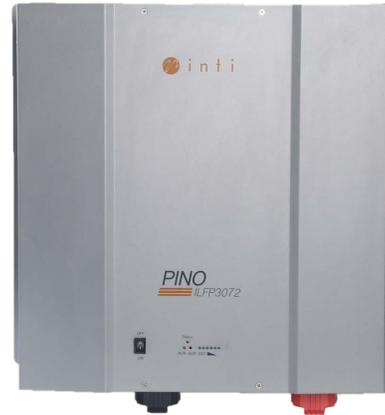
Inti's Pino is a maintenance-free LiFePO4 lithium ion battery with a diverse range of nominal capacities at 25.6Vdc and 51.2Vdc, and with a lifetime of  $\geq 3\ 650$  cycles at 80% DOD and 25°C. The customized battery charging system with integrated smart BMS with temperature protection and RS485 type communication allows for extended battery life.
