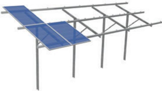
Ground mount system, single-base with support, two rows of modules, vertical installation
