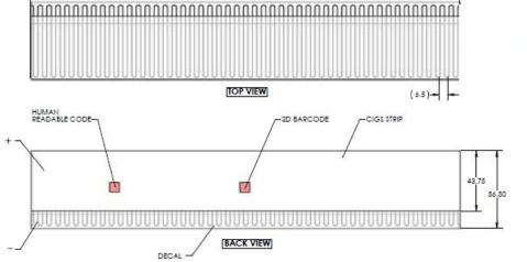
Thin-film CIGS solar cells on stainless steel substrate have high efficiency levels and provide significant advantages over conventional, rigid solar cells.
