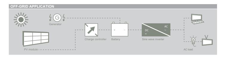
The inverter converts the DC battery voltage (direct current) into 230V<sub>AC</sub> (sinusoidal alternating current). Voltage-controlled, it provides a stabilized, quartz-precise direct current of 230V<sub>AC</sub>/50Hz (other voltages and frequencies as per type label).
