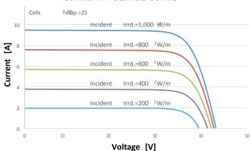
rrent-voltage characteristics with dependence on irradiance and module temperature
