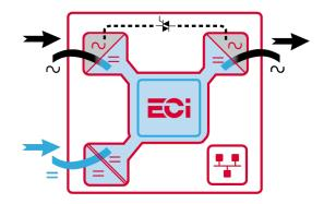
The ECI technology eliminates all single points of failure with full scalability; up to 32 modules in parallel and high efficiency of up to 95% in AC to AC conversion, and above 93% in DC/AC conversion, hence reducing operating costs.
