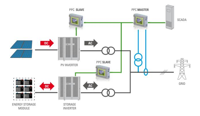
The FIMER transformerless MV CENTRALIZED STORAGE INVERTER is a bidirectional three phase inverter specifically designed for implement storage solution in large-scale PV plant and MV connected installation.
