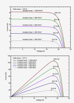
STC: Irradiance 1000W/m<sup>2</sup>,Module temperature 25°C,AM1.5 spectrum.
