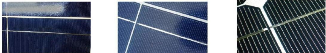
Figure 6 : Some common compatibility problems ( EVA with solar cells、flux、backsheet and glass )
