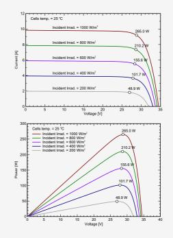
STC: Irradiance 1000W/m<sup>2</sup>,Module temperature 25°C,AM1.5 spectrum.
