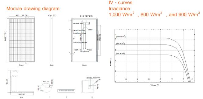
These data represent the performance of typical modules as measured at their out put terminals, and do not include the effect of such additional equipment as diodes or cables. The data are based on measurements made in accordance with ASTME 1036-85 corrected to SRC (Standard Reporting Conditions, also known as STC or Standard Test Condition), Which are :
