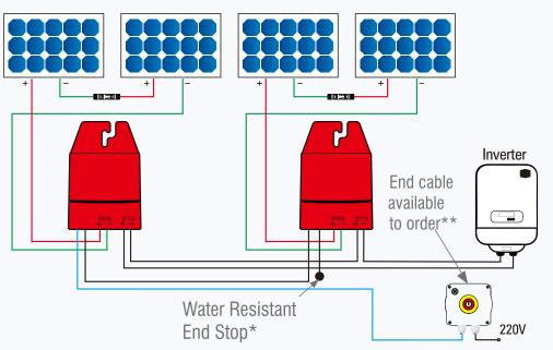
Each BFS-11 device operates two solar modules, the modules in series go to inverter sting as usual. The only difference is the communication signaling cables connect the BFS-11 in series and go to the button switch complete the RSD solution.
