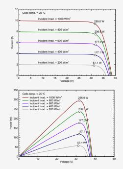
STC: Irradiance 1000W/m<sup>2</sup>,Module temperature 25°C,AM1.5 spectrum.
