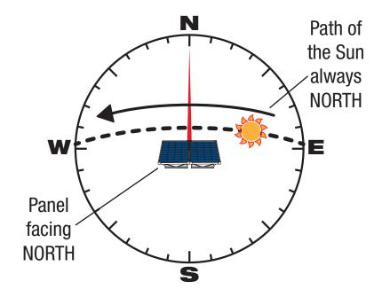
The optimal angle from ground of the panel is around 30°. Anywhere between 10° and 40° ensures good power generation across the course of the day.
