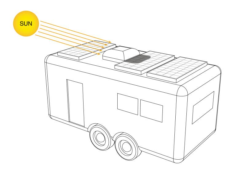
Be aware of shading that can occur as a result of roof mounted accessories on your caravan or motorhome. Shading sections of your solar panels will significantly reduce your solar panels performance. Care must be taken to avoid the possibility of shading as much as possible during the installation process.
