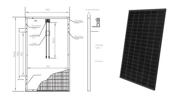
Module dimensions in the technical picture are expressed in mm with tolerance +2 mm (+007V ') 1 - Standard Test Conditions (STC) imadiance 1000 Wim/ Air Mass AM - 15. Cell Temperature 25°C2, Power measurement uncertainty within + 3%. 2 - AEG photoothics modules are classified according to a pincipide of positive power bleance: the Power Output measured at STC of the delivered modules exceeds their assigned Nameplate Nominal Power at STC. ertainty within ± 3%.
