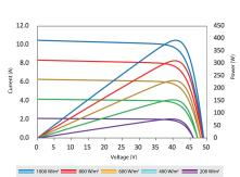
Current-Voltage & Power-Voltage Curves At Different Irradiances
