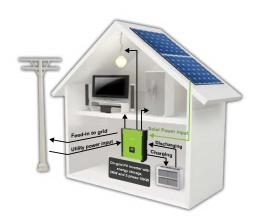
Feed-in is not the only choice In comparison with conventional grid-tie inverter, EHCS-LV can not only feed-in power to the grid but also store solar power to the battery for future usage and directly power to the loads.
