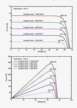
STC: Irradiance 1000W/m<sup>2</sup>,Module temperature 25°C,AM1.5 spectrum.
