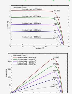
STC: Irradiance 1000W/m<sup>2</sup>,Module temperature 25°C,AM1.5 spectrum.
