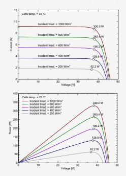
STC: Irradiance 1000W/m<sup>2</sup>,Module temperature 25°C,AM1.5 spectrum.
