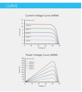
Note: the specifications are obtained under the Standard Test Conditons (STCs): 1000 W/m² solar irradiance, 1.5 Air Mass, and cell temperature of 25°C. The NOCT is obtained under the Test Conditions: 800 W/m², 20°C ambient temperature, 1m/s wind speed, AM 1.5 spectrum.
