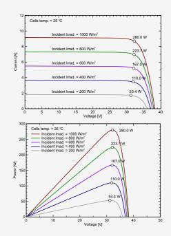
STC: Irradiance 1000W/m<sup>2</sup>,Module temperature 25°C,AM1.5 spectrum.
