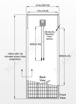
Dimensions in brackets are in inches. Un-bracketed dimensions are in millimeters. Unit: mm[in.]
