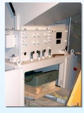
An accurate classing of the cutting material can be enabled by installing a granulate screen underneath the cutting unit. The screen hole size will be adapted to the according request. Chips with screen size pass the sieve and fall into the deposit device, oversize chips get back to the cutting zone.
