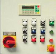
The operation panel at the electrical cabinet contents all relevant operation elements, which allow a reliable operation. The personnel security is assured by security switches on revision openings to prevent against unauthorized access into the cutting zone.
