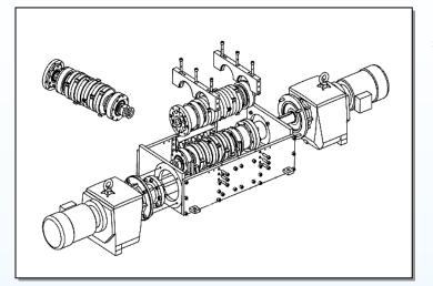
Enabling the lift-out of the entire cutting shafts, the divided frame of the cutting unit allows a fast exchange of the cutting unit, if requested.
