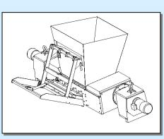
Inside the feeding funnel a mechanical, electromotive or hydraulic driven pushing device can be installed to enable a continuous operation even with problematic-to-handle cutting material.
