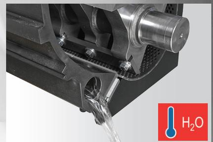
Grinding chamber water cooling; screen surface equal to approximately 50% of knives rotation length.
