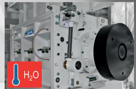
Water cooling system of the grinding chamber.
