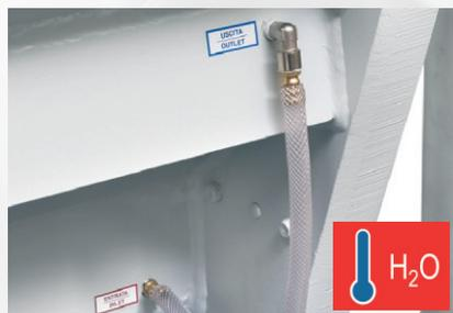
Grinding chamber water cooling. Surface screen equal to approximately 50% of knives rotation length.
