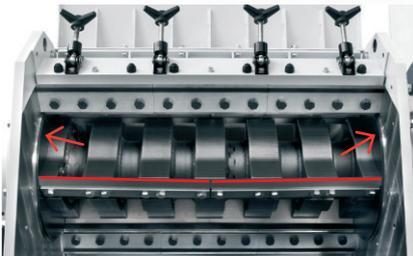
Rotary discs integral with the rotor and rings. Arrow cutting configuration for grinders with 3 or 5 knives; bench adjustment of rotating and fixed knives.
