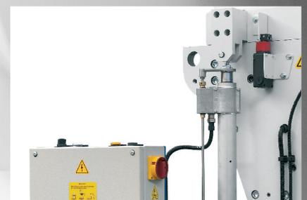
Hopper opening with motorized jack and screen-holder opening by gas cylinder.
