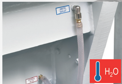
Grinding chamber water cooling. Screen surface equal to approximately 50% of knives rotation length.
