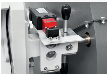
Rotor lock for maintenance. Safety devices and circuit in compliance with EEC Directives.
