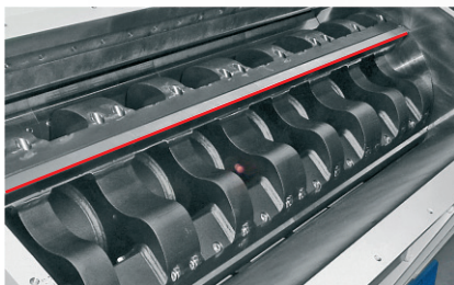
Scissors cutting configuration for 5 knives rotor. Bench adjustment of rotating and fixed knives.
