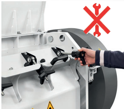
Access without tools to the parts subject to ordinary maintenance.
