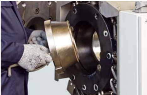
Easy replacement of the die plate
