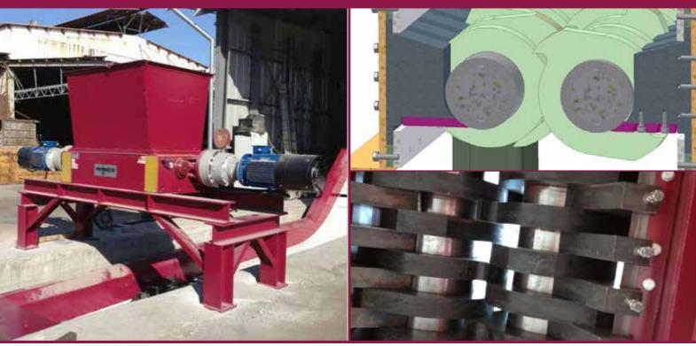
The cutting discs are designed according to the material to be processed and the kind of shredding, thus defining the thickness and the disc diameter over the geometry of the hooks. Equipped with rotor's cleaning knives
