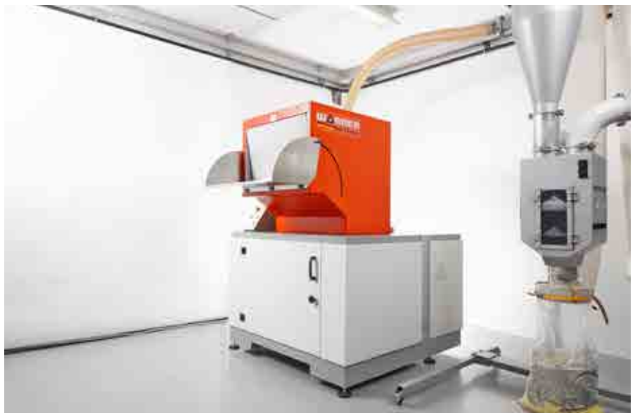
Wanner E45.80 with integrated blower, cyclone separator and dedusting system. ▶
