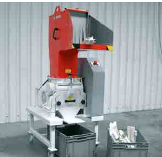
D 25.25 Granulator on central granulating stand, in this case used for grinding extruded profile cuttings.
