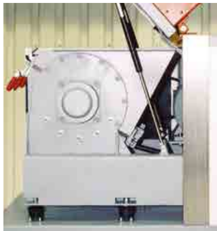
The large cutting chamber with V-shaped rotor is easily accessible.
