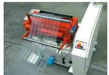
D25.50 Granulator with roller infeed for processing sheet and trimmings.
