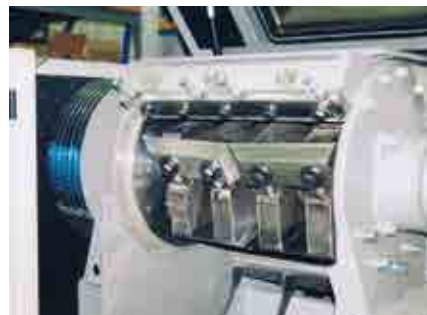
The large cutting chamber with V-shaped rotor is easily accessible.
