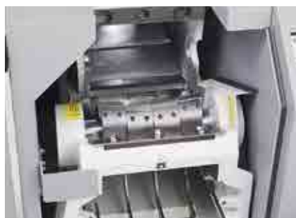
Cutting chamber easily accessible without tools.
