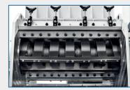
3 or 5 knives rotor with scissors-cutting
