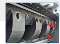
Keys for the fixing of motor pulley and flywheel Pulley and flywheel manufactured as per drawing
