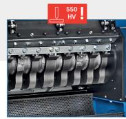
Grinding chamber in anti wear execution
