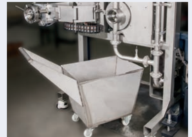
Very good accessibility underneath the pelletizing unit and the polymer diverter valve
