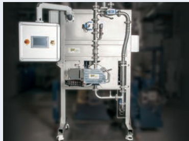
Machine base frame with castors to support the pelletizing unit and the control panel
