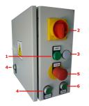
1. The green light "POWER" indicates a connection of the bale to power and that the main switch is turned ON
