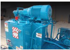
Marathon's advanced power pack is designed so that all the valves are contained in a single manifold, which minimizes the number of hose connections.
