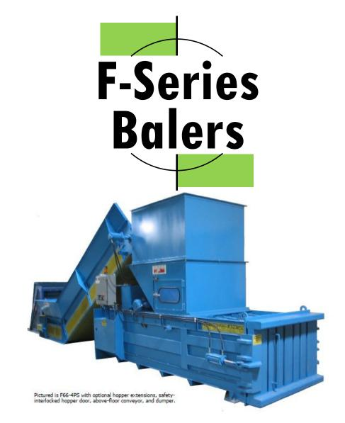
F-Series balers from Summit Equipment, Inc. are engineered for peak performance in baling OCC, ONP, CPO, office paper, UBC, and tin cans. They can also be modified for plastics, foam, and other special materials. Bales are sized to an industry-standard 30"H × 48"W × 60"L and will weigh 900-1200 lbs in OCC.
