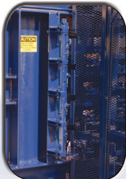
New Hinged Side Rails and Redesigned C-Clamp Produce Bales With High Integrity and Easy Escapement
