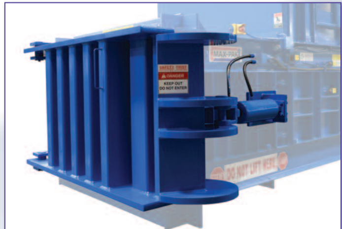
The massive door clamp is hydraulically operated and secures the baler door with an extra measure of safety, by transferring the packing forces through the baler frame and body.
