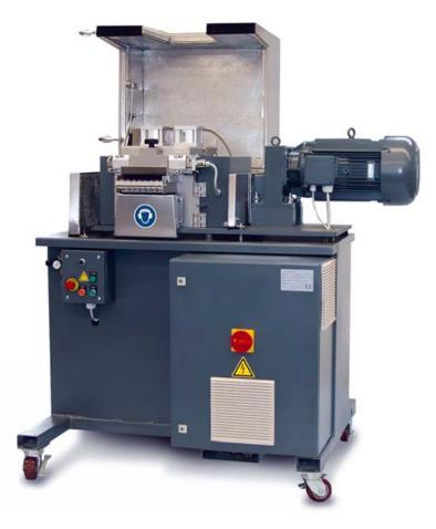
Supported in bearings on both sides, the BAOLI dry-cut strand pelletizer produces cylindrical pellets of excellent quality ideally suited for further processing. BAOLI offers three machine sizes with working widths of 100 mm, 200 mm and 300 mm for pelletizing up to 75 polymer strands. Its modern cutting tools guarantee high throughput levels and provide long-term availability of the strand pelletizer.
