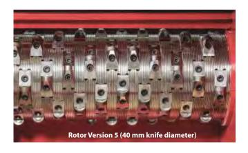
The highly efficient scissors cut of the concave ground circular cutting heads provide a very high work rate with very little effort. The knife holders are welded or mounted on the rotor and the round knives can be turned up to **8 times** with just a few adjustments before having to be exchanged completely. The use of various types of knives enables jobrelated adjustment of the shredder to the material being processed.
