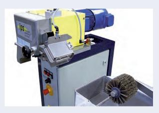
Strand feed guide with integrated strand dewatering by blowing (ips-SG-E 30 Kombi)
