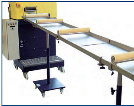
Strand feed from strand cooling trough to strand pelletizer
